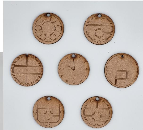
Laser cutting MDF prototypes made me realise that a watch would be difficult to design a screenless interface for due to dimensional constraints. Thus, I developed larger PLA 3D printed prototypes that could clip onto a pocket, belt, bag, or keychain. This increased versatility and made the interface easier to design in a way that is understated rather than absorbing.
