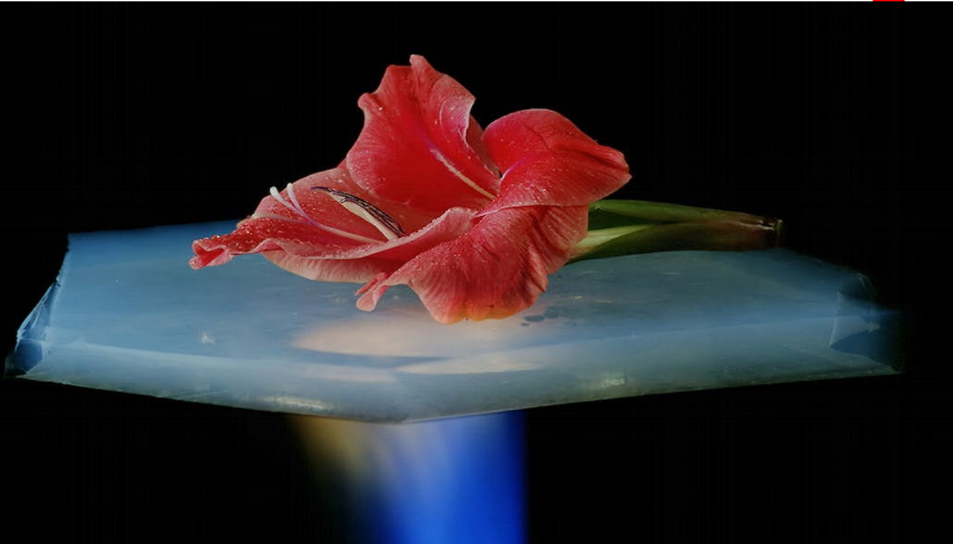
Aerogel insulating a flower from the heat of a Bunsen burner
