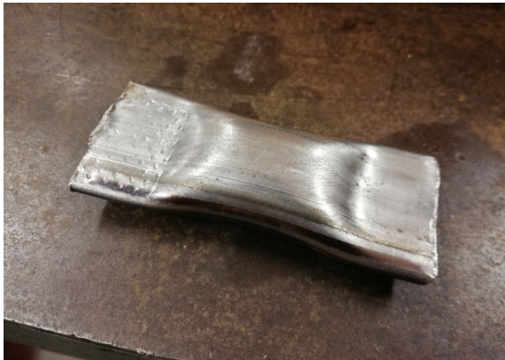
Metal support bar flattening test comparing directly placing steel tube in the vice (leaving indentations) versus wrapping it in a leather glove for a smooth edge.
