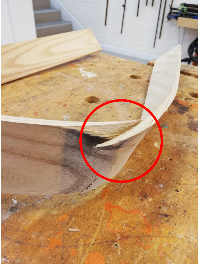
FAILED - 6mm ash freehand test bend fractured due to insufficient time steaming and tightness of radius without a jig.
