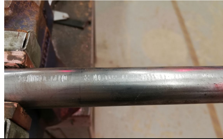
Vice indentations on tubular steel when filing corners – needs filing and a finish to cover surface imperfections.
