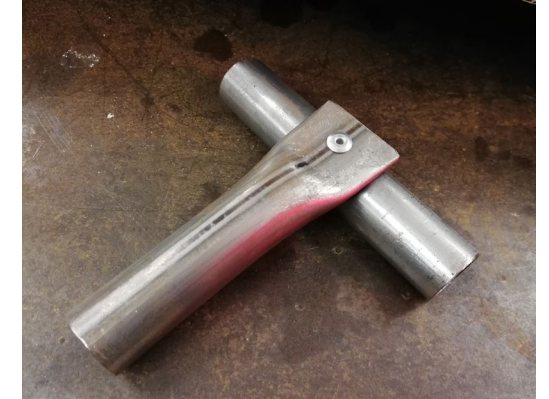
Metal-to-metal rivet test without washers demonstrates a clean aesthetic and a quick connection method.
