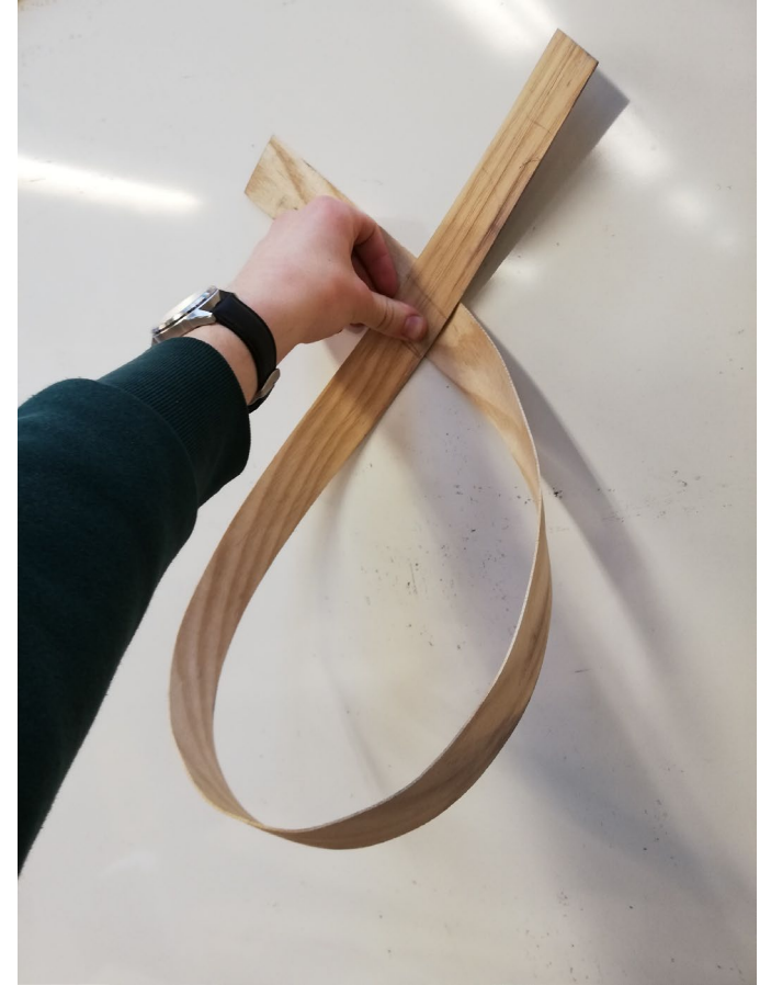
SUCCESSFUL - 1.5mm ash freehand test bend of curved lampshade structure
