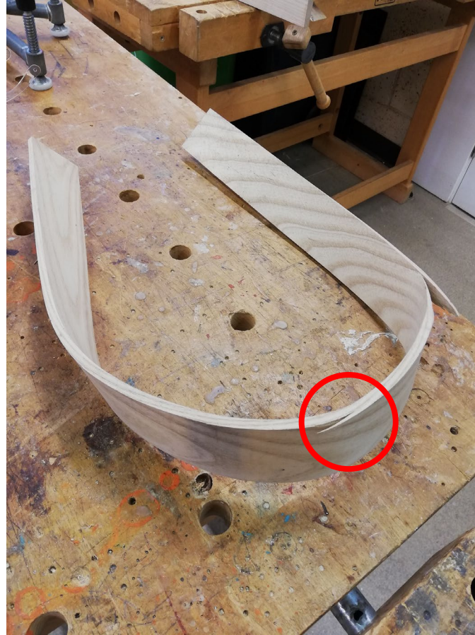
FAILED - 6mm ash freehand test bend fractured due to insufficient time steaming and tightness of radius without a jig.
