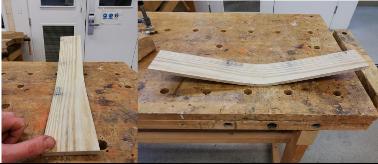
FAILED – 9mm slat test bend. Jig broke under spring-back pressure causing distortion. The bend is also too sharp for an ergonomic seat.
